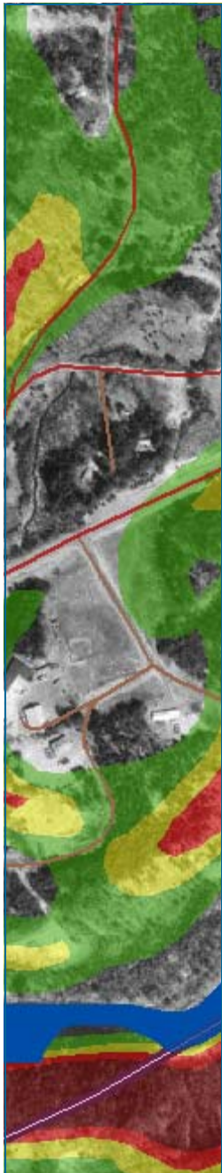
Multicriteria spatial decision support for NERON. Potential locations for new NERON sites shown in dark green. Selection criteria in this example includes proximity to roads, slope, and avoidance of conservation lands and water.
